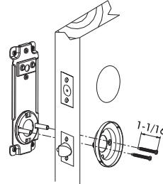
Place outside knob assembly against door face with square spindle engaged with latch square drive. Insert two horizontal mounting screws from inside and tighten.
