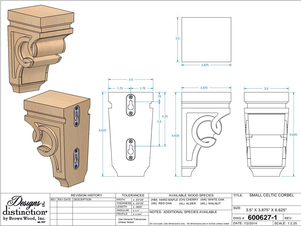
PROPRIETARY AND CONFIDENTIAL THESE DRAWINGS AND SPECIFICATIONS ARE THE PROPERTY OF BROWN WOOD INC. AND ARE ISSUED IN STRICT CONFIDENCE AND SHALL NOT BE REPRODUCED OR COPIED OR USED AS THE BASIS FOR THE MANUFACTURE OR SALE OF APPARATUS WITHOUT PRIOR WRITTEN PERMISSION.
