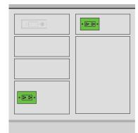
Do NOT put the electrical supply directly behind the drawer box as it may interfere with the cable management arms
