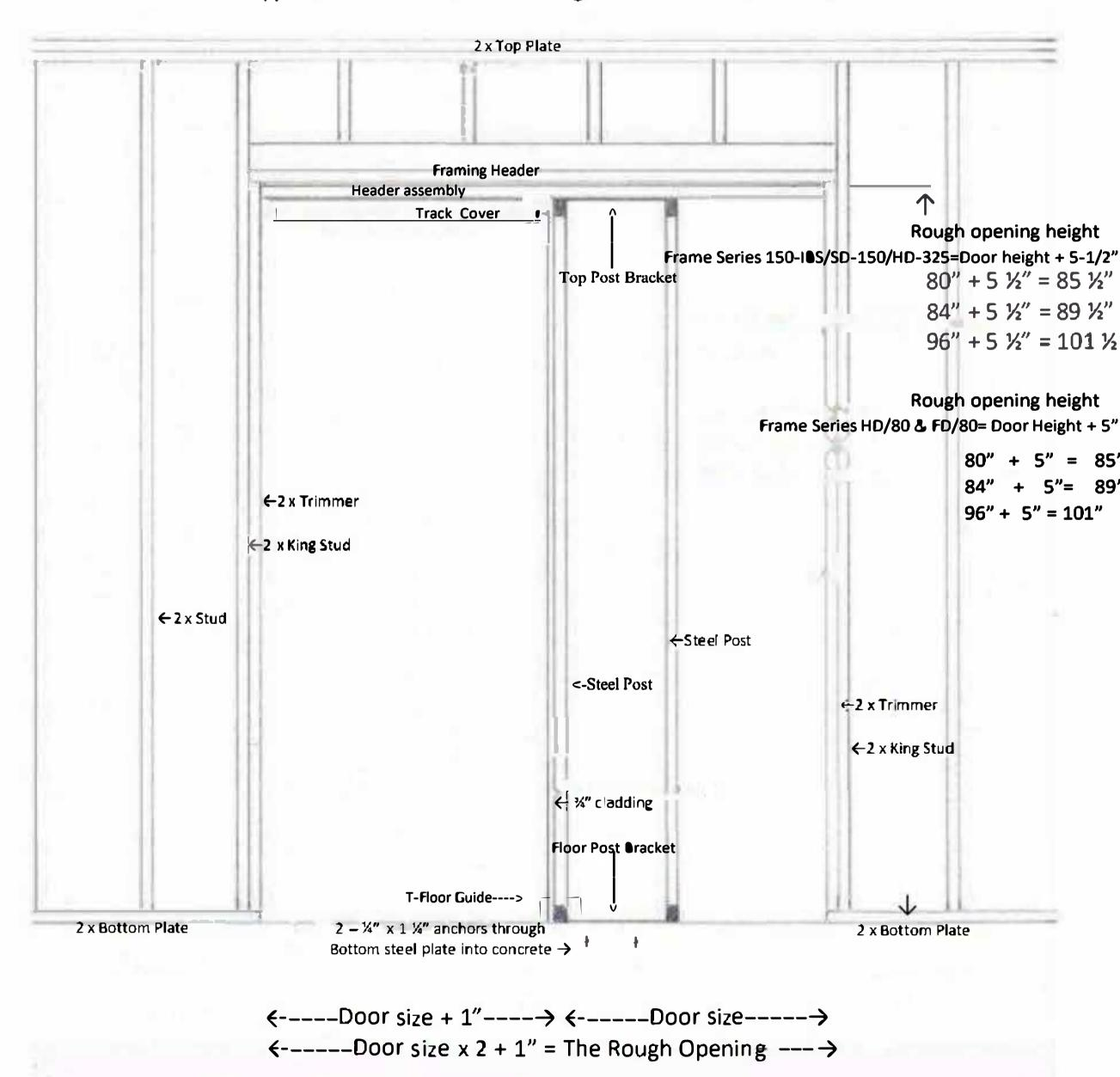
HDPOCKETDOORS fabricates standard sizes of heavy duty pocket door frames for 2x4 and 2x6 walls for 80", 84, and 96" door height and 48" (and smaller) door width. With ample lead time, custom frames can be available for any height, width, wall thickness for any application.
