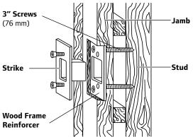
Furnished with standard and round corner deadbolt strikes, this reinforcer significantly strengthens a jamb against "kick-in" attack and greatly increases the security of the lock. The reinforcer is concealed under the strike and is anchored to the jamb with two 3" long screws. B500 Series metal dust box reinforcer anchors (B520-622) to jamb with three 3" screws.
