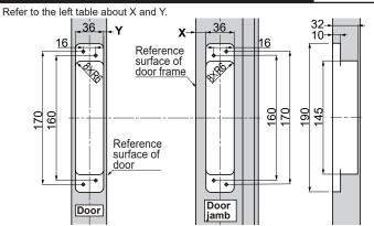
When not using the installation template HES3D-W190-TMP (sold separately) drill pilot holes at the installation screw locations."
