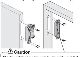
Before installing base frame into the Doorjamb, check that it is oriented correctly. If the orientation is incorrect, the door cannot be installed.
