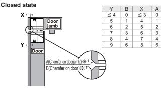
\* 1 Chamfer is needed depending on the amount of X and Y.
