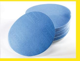
Whether you are sanding hardwood, softwood, particle boards, lacguer or veneer, Ekablue is your go to choice for a wide range of applications. Manufactured on a lightweight latex paper, the durable, precision coated aluminum oxide grain ensures superior life and quality finish with a fast and consistent cut. Experience the power of the blue now!
